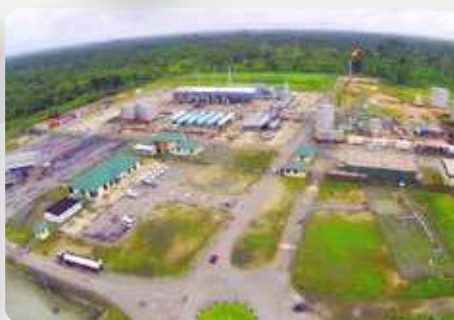
2015 The addition of the 1000bbls/d Mini Refinery and 100MM Scf/d capacity Gas Processing plant.
